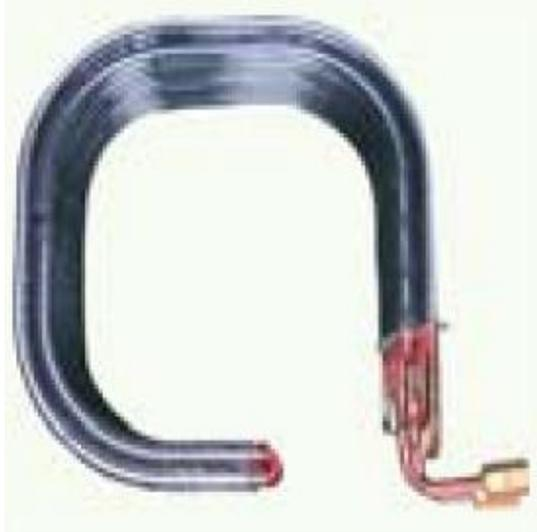
"C" type exchanger is helpful to improve the well-distributed of terminal air duct and refrigerant system, make the efficiency of multi flow more even and it reduced the probable of system leak. Blue fin extremely reduced the coagulate water detained in the aluminum flake, so it reduce the air resistance, improved the efficiency of heat exchanger.
